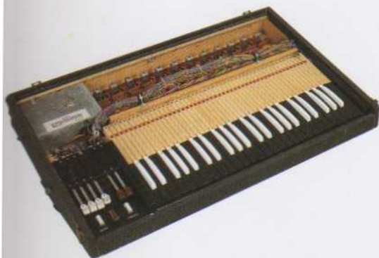
The inside of an early Vox Continental organ with orange top removed, showing how at this period the instrument had wooden keys. Later examples had plastic keys and modified electronics, giving a different feel and sound.
