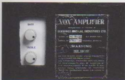
Some Vox AC-30 amps featured this treble-enhancing "top boost" circuit fitted to the rear.
